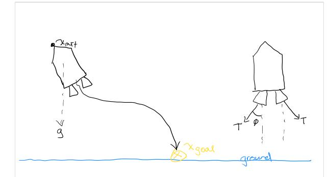
p: can't angle (angle between thruster and vertical)
